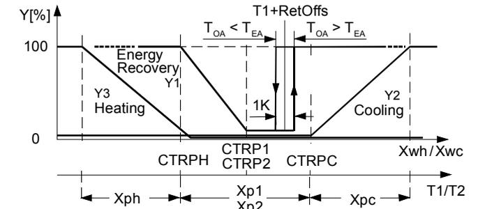
A fixed hysteresis of 1K is used, to switch between 0% position and actual Y1 signal.
