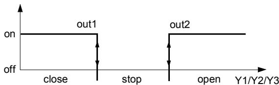
An automatic synchronization function ensures correct positioning of the actuators. This is performed by running all actuators to the closed position periodically. The run time for synchronization is derived by control parameter **RuntimeYx** (x = 1, 2 or 3) multiplied by 1.25.
