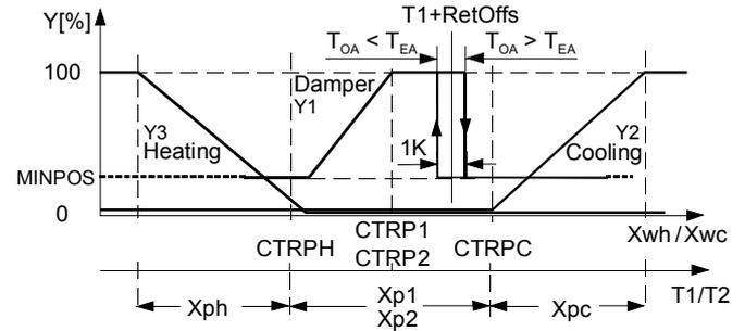
A fixed hysteresis of 1K is used, to switch between **MINPOS** and actual Y1 signal.
