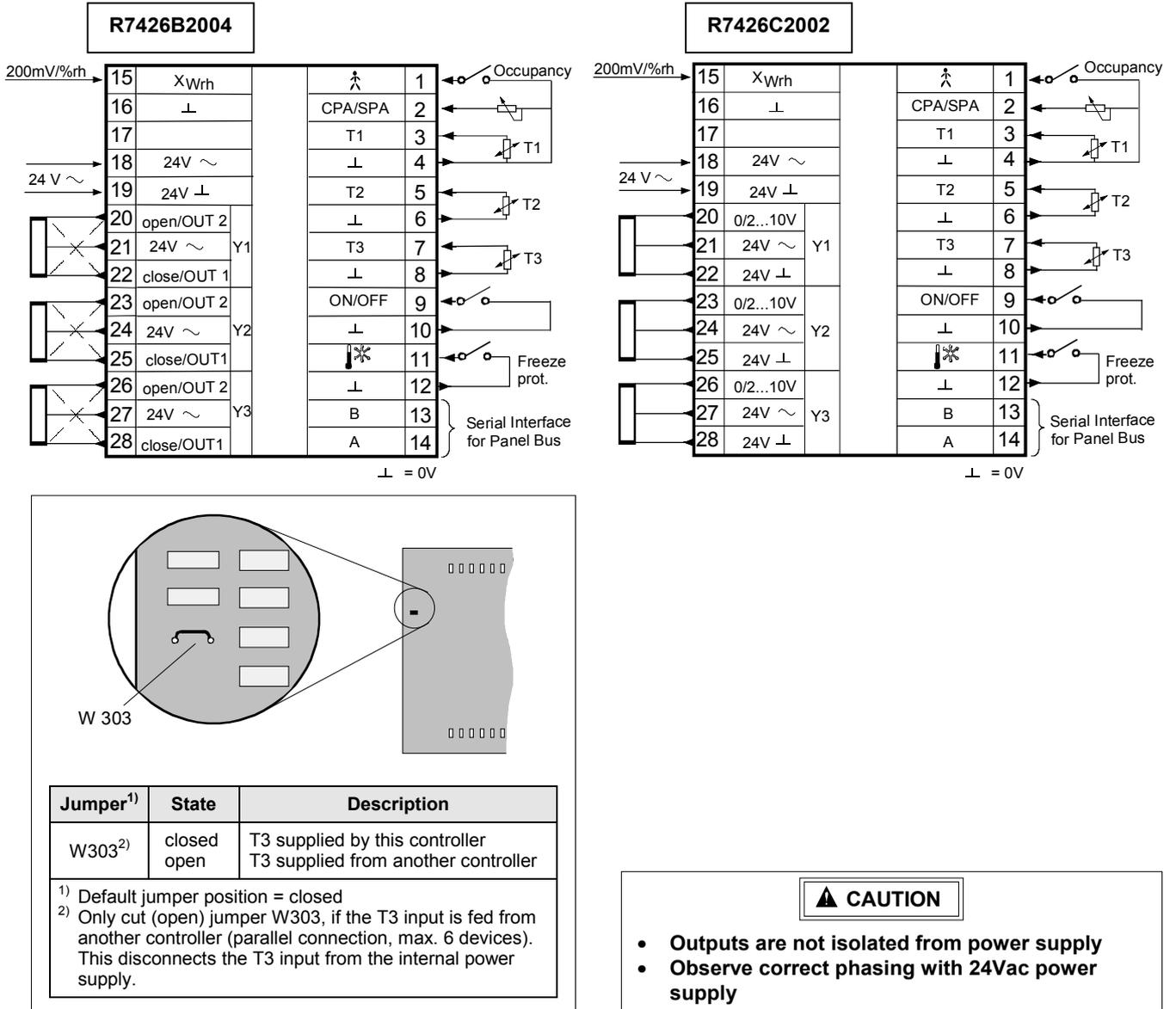
Fig. 3. Connections and Jumper coding
