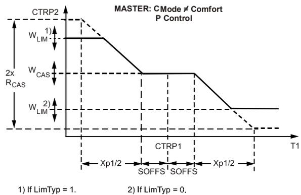
Low limit of CTRP2 is performed if control parameter **LimTyp** = 0 and high limit of CTRP2 is performed if control parameter **LimTyp** = 1.
