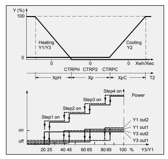
**Time Control.** Depending on the programmed time schedule of the internal controller real time clock the different operating control modes Comfort, Standby, Night or OFF are selected. In the OFF operating mode the controller automatically switches OFF the selected number of heating stages/steps, closes the cooling valve (5b), switches the fan(s) OFF and thereby closes the dampers (6) by an external installed relay logic.
