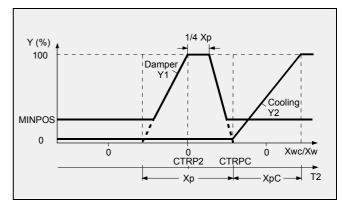
corresponding to the 0...100% correctional signal to reposition the mixed air dampers (6) or cooling valve (5) to maintain the desired discharge air temperature. The minimum outside air damper position adjustment (MINPOS) on the controller determines the position to which the outside air damper will be driven even though the temperature input condition demands that it should drive to the fully closed position.
