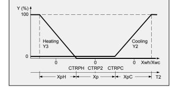
the desired internal calculated setpoint. If a deviation between the two values exists, the controller generates two 0(2)...10Vdc control signals in sequence via outputs Y2 and Y3 corresponding to the 0...100% correctional signal to drive the electric current valve (5a) for proportional control of the electric air heater or to reposition the cooling valve (5b) to maintain the desired discharge air temperature.
