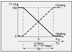
Cascade Temperature Control. The return or room air temperature sensor (1a, b or c) measures the actual value and the controller (4) compares this value with the de-
