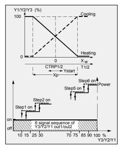
Time Control. Depending on the programmed time schedule of the internal controller real time clock the different operating control modes Comfort, Standby, Night or OFF are selected. In the OFF operating mode the controller automatically switches OFF the selected number of stages/steps and the fan(s) and thereby closes the dampers (6) by an external installed relay
