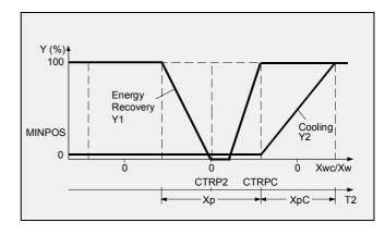
the energy recovery valve (5b) or the cooling valve (5a) in sequence to maintain the desired discharge air temperature.
