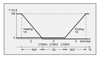
between the two values exists, the controller generates a 3-position control signal to reposition the heating or cooling valve to maintain the desired discharge air temperature.
