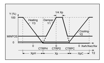
corresponding to the 0...100% correctional signal to reposition the mixed air dampers or heating or cooling valve to maintain the desired discharge air temperature. The minimum outside air damper position adjustment (MINPOS) on the controller determines the position to which the outside air damper will be driven even though the temperature input condition demands that it should drive to the fully closed position.
