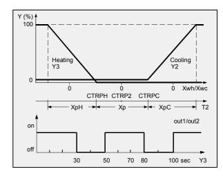
3-position control signal on output Y2 to reposition the cooling valve (5b) to maintain the desired discharge air temperature.
