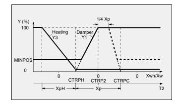
corresponding to the 0...100% correctional signal to reposition the mixed air dampers or the heating valve to maintain the desired discharge air temperature. The minimum outside air damper position adjustment (MINPOS) on the controller determines the position to which the outside air damper will be driven even though the temperature input condition demands that it should drive to the fully closed position.
