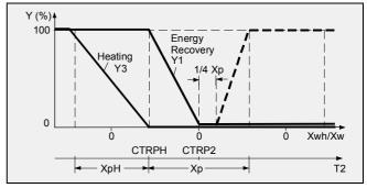
The discharge air temperature sensor (2) measures the actual value and the controller (4) compares this value with the desired internal calculated setpoint. If a deviation between the two values exists, the controller generates a 3-position control signal on outputs Y1 and Y3 to reposition either the energy recovery valve (5a) or the heating valve (5b) in sequence to maintain the desired discharge air temperature.
