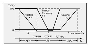
heating valve (5a) or the cooling valve (5b) in sequence to maintain the desired discharge air temperature. If the actual temperature is below the setpoint, the controller modulates first via output Y1 the heat recovery valve (5c) into the open position and if fully open, the heating valve (5a) is opened in sequence via output Y3. If the actual temperature increases the sequence of operation is reversed.
